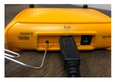
3 – While holding in the black button with the paper clip, simultaneously plug the Base Station back into the laptop computer.
