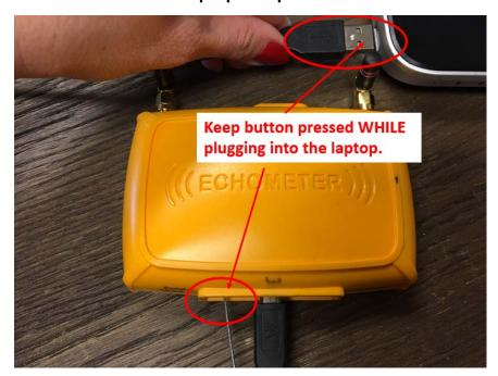
4 – The Base Station Status light should turn full on Green, indicating a programming status. Step through the following prompts within the TAM software to reset the Base Station.
