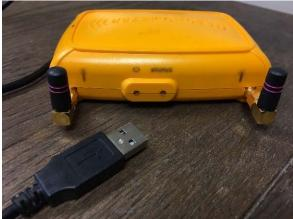
2 – Using a paperclip or similarly sized object, Press and hold the black recessed button to the left of the USB cable insert.
